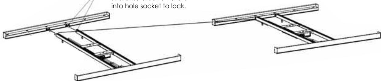
**Note the direction when installing; the driver tray is on top when the fixture is hung.**
