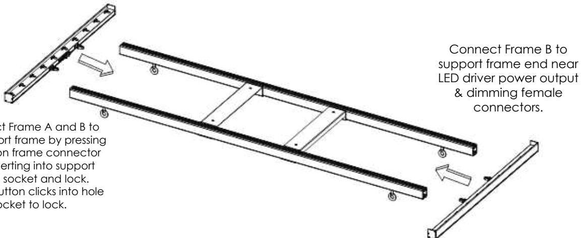
**Note the direction when installing; the LED driver mounting bracket is on top when the fixture is hung.**
